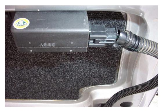
At the top left (by the little lotus badge) is a small mechanical arm of about 1" long. When the button is pressed it retracts into itself. This has an eye much like a needle. Loop one end of the bike brake cable through this eye and the other end is looped through the small hole on the bottom of the boot lock mechanism.
