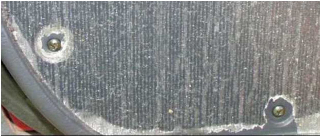
close up of screws removed, on left side of handle, and you can see the two others to remove on the right hand side , note they have washers behind them, watch out they don't fall as you remove the bolts. A tip for when putting them back on is to get some sticky glue to hold them, pritt stick works fine.
