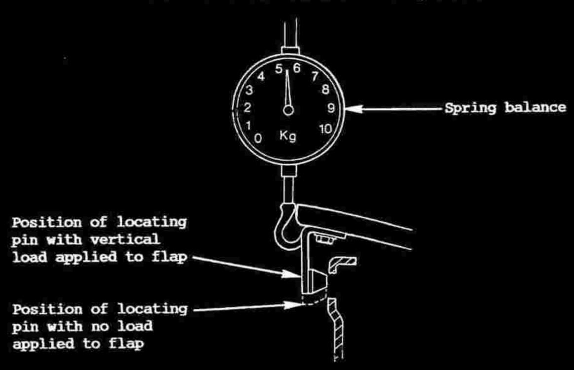
If the pin is too high, adjust the four flap upstops \ turn counterclockwise and recheck. Recheck operation with no flap loading.
