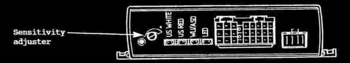
Adjustment Procedure: Turn off the siren (using the siren key), and use the hazard lamps as an indication of alarm triggering.
