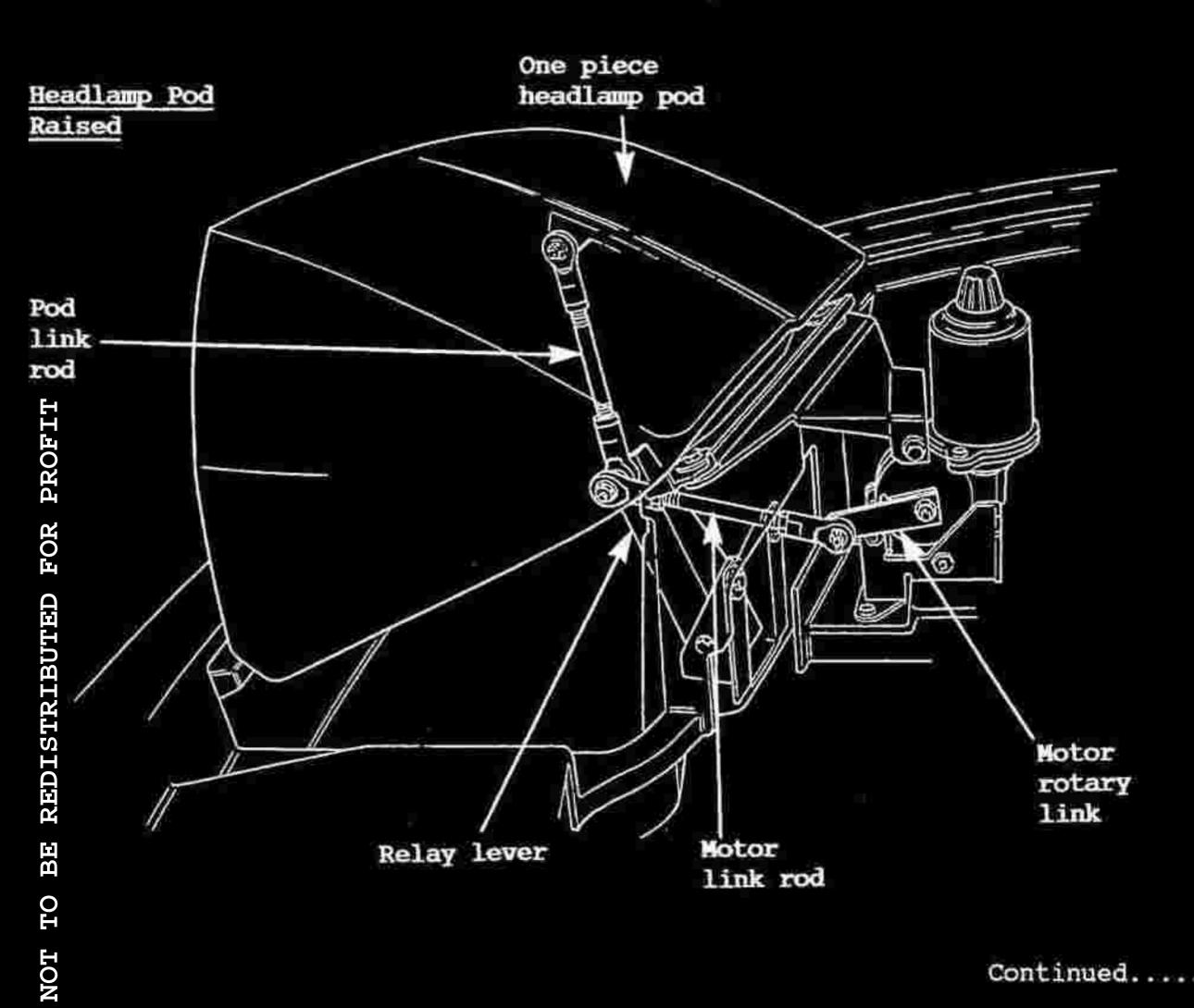
Operation: When the headlamps are switched on, the headlamp motor operates and the rotary link moves forwards until it contacts the upstop, when the motor stalls and switches off. In the up position, the pod link and the relay lever form an almost straight load path to hold the pod steady. Electrical control is similar to the previous system except that:
