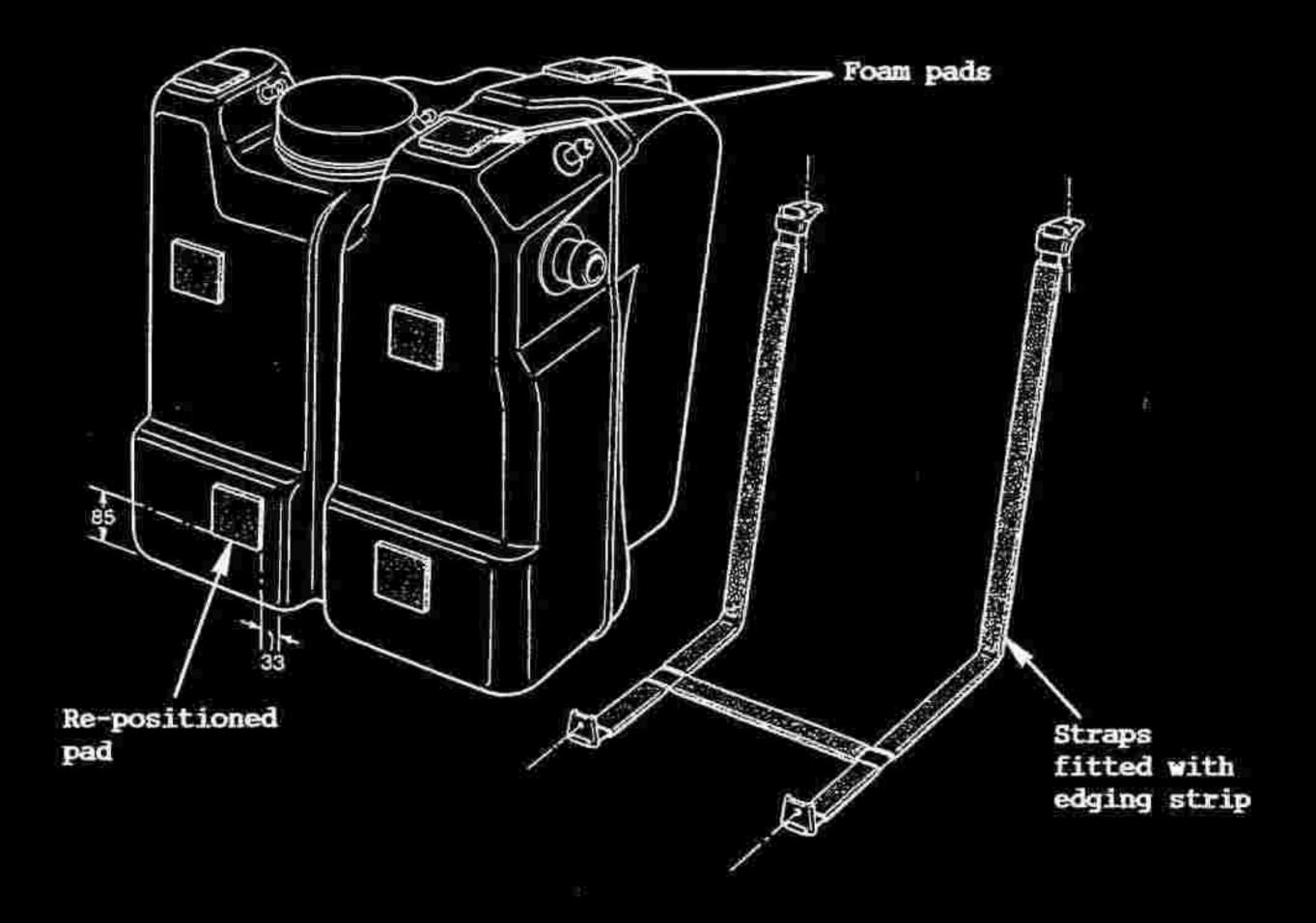
Refit the tank in the reverse order to removal;
