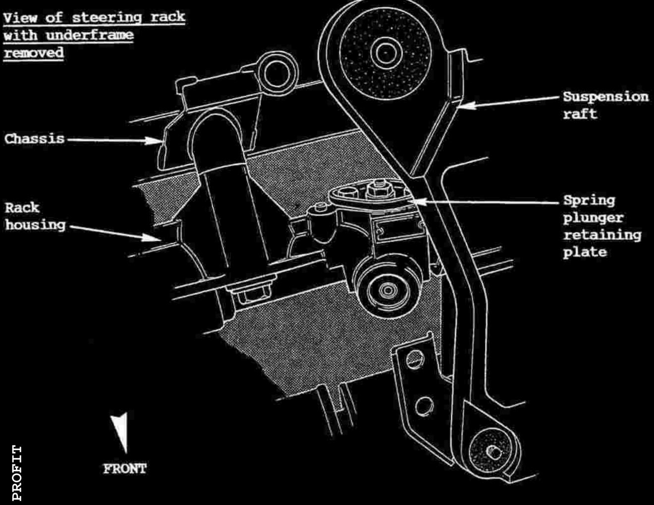
5. Refit the spring and spring cup, and check that the sealing ring is correctly positioned on the rack housing before fitting the retaining plate with its two screws and shakeproof washers. Torque tighten the two fixings to 23 Nm (17 lbf.ft).
