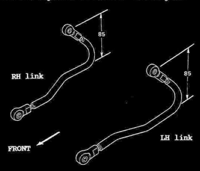
If operation of the existing headlamp mechanism is satisfactory, it is necessary to adjust only the cover flap upstops and 'J' links as detailed from step 7 of the following set up procedure. First remove the cover flap outer panels and screw the flap upstops fully down.
