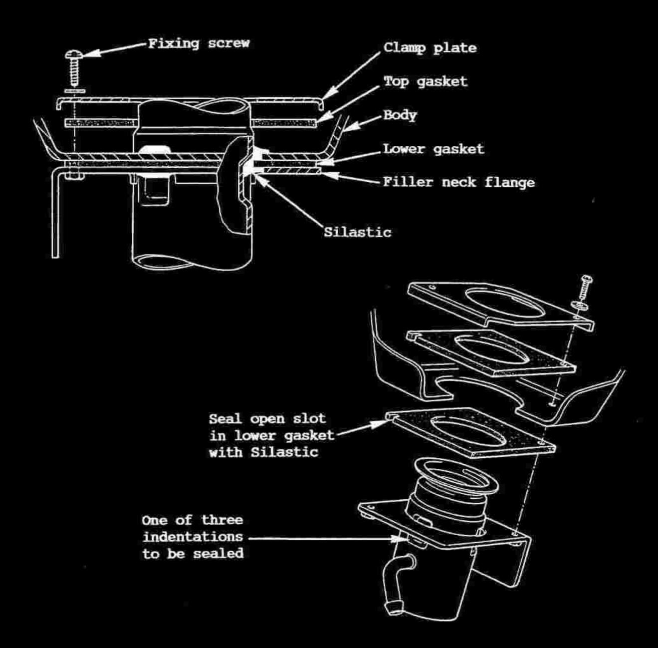
Remove the filler flap catch from the body, and apply black Silastic to the whole of the catch flange before refitting. Remove the filler flap hinge fixings, and reassemble using a rubber washer (A082W4115F) between the flat washer and inside of the body.
