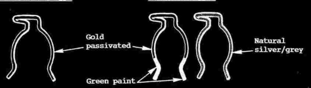
If non preferred type clips are found to be fitted at the transmission end, it should be assumed that these also will be fitted at the gear lever end, and all four clips should be replaced with preferred types (A100F6060F).
