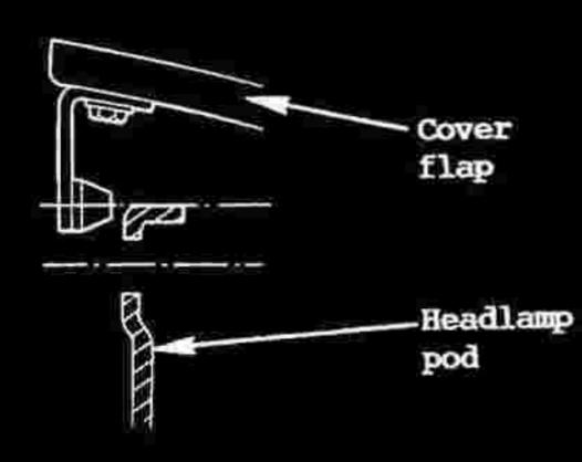
Wind down the pod. Apply one full turn counterclockwise to the flap outermost upstops, and a half turn counterclockwise to the innermost upstops. Tighten locknuts.
