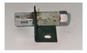
First step, dismantling...the valve is made up of three main hexagonal sections (D, E & H), these all simply screw together. Separating the two larger sections (E & D) will release the mounting bracket and reveal the large sealing ring (A). This seal is normally serviceable as it is not a moving part.
