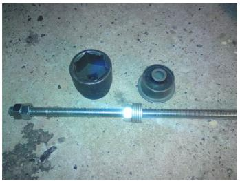
Lightly oil the threads on the free end of the bar, and slide on the socket, and the bush...
