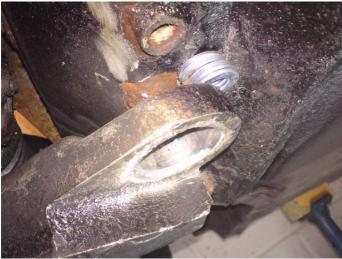
Lock two M12 nuts against each other at one end of the threaded bar, with a third nut about 100mm further along with a few washers to aid turning...
