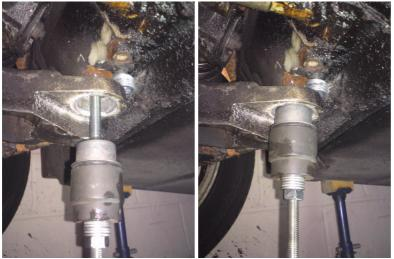
Once the start of the bush is bought up to the casting, double check that all is lined up well.
