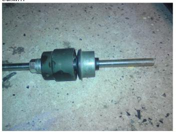
Offer the bar into the bush hole, and screw into the chassis – at least 25mm, using the locked nuts...
