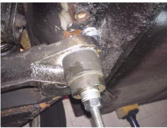
Be sure to get the flange of the bush fully flush with the raft casting. Once you're happy it's home, loosen the tension on the single nut, then using the locked nuts, wind the whole tool back out of the way...
