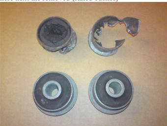
The failed bushes were pretty easy to remove, by driving a chisel into the side of the outer sleeve, causing the sleeve to collapse – done carefully, this caused no damaged whatsoever to the casting of the raft.
