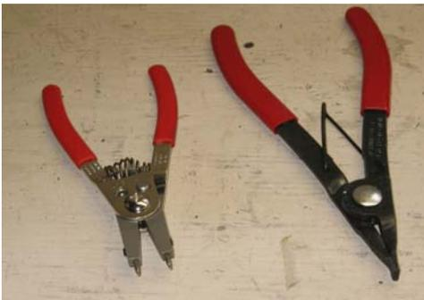
Internal snap ring pliers (smaller pair) are used to compress the retaining ring before removal and reinsertion into the piston cylinder. External snap ring pliers (larger pair) are used to expand the locator ring for insertion around the piston itself
