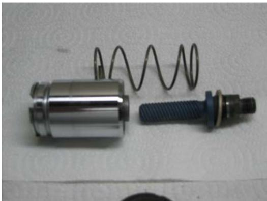
Brake piston, actuator screw and return spring, after cleaning.
