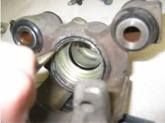
If the retaining ring doesn't come out when you pull off the boot, remove the retaining ring from the caliper cylinder with the needle nose pliers. This was one of the more frustrating steps, as the retaining ring had been pressed flush against the cylinder wall by years of pressure and was virtually indistinguishable from the cylinder wall.
