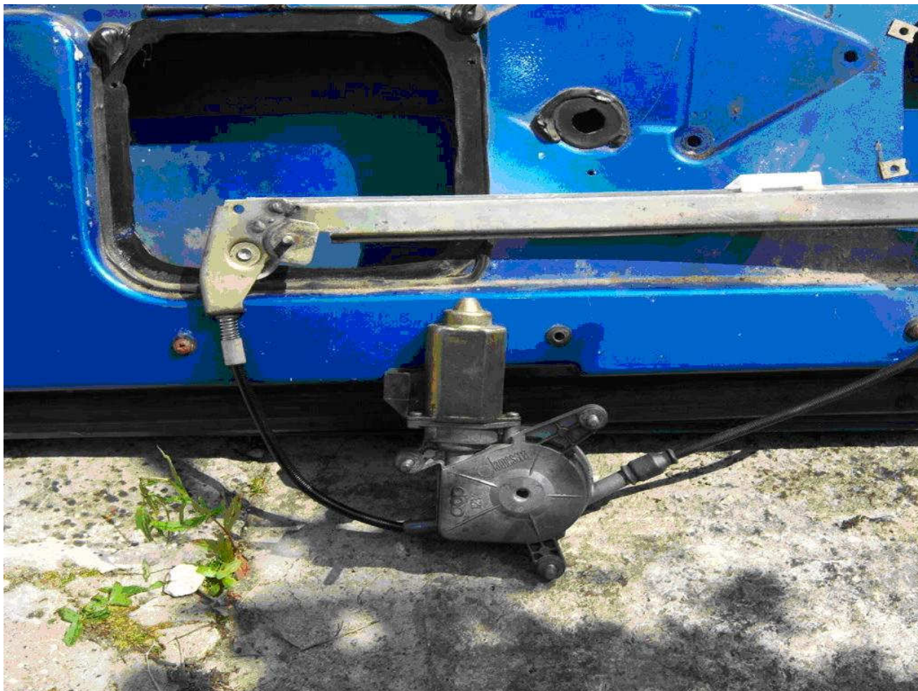
3) Squash it down a bit, and slide it in via the speaker aperture
