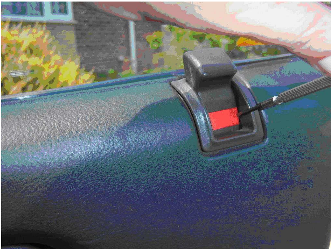
7) Remove the screw on the trailing edge of the door card
