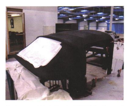
2) Canopy folded showing highlighted are of pressure caused by frame.
