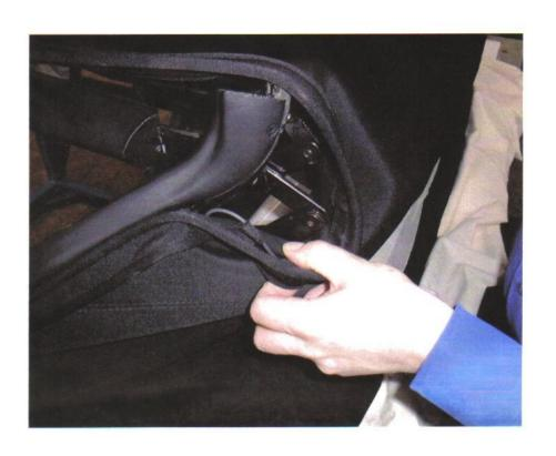
8) Stand at rear of vehicle and make sure canopy is pulled clear of linkage before folding into stowage position.
