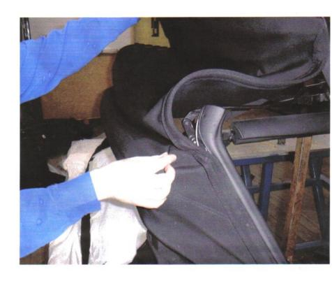
4) Slide canopy over linkage to relieve pressure on material.
