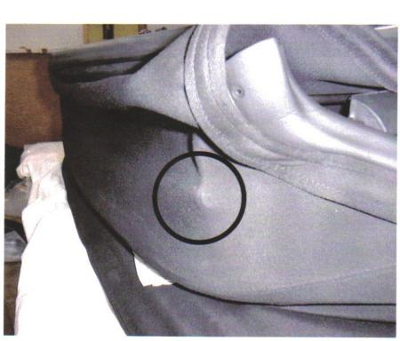
3) Picture showing area on canopy when partially folded that needs moving to prevent fouling on canopy
